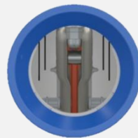
Neutral position Switch OFF. Change-Over Switch in earth position.
